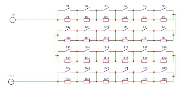
Above: QR101 relay-resistor network schematic (while number of QR100 base resistors is 14). The algorithm is to selectively control the opening and closing of the switches/relays (S1~S24) to selectively pass or shield the base resistors (R1~R24), thus outputting the resistance value (PV) that is closest to the set value (SP). The nominal step value is determined by the smallest base resistance value, and the device cannot perform a scanning output with a smaller step.
