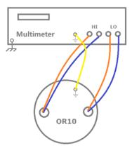
It should be reminded that the distortion of the power supply waveform and noise may also have an impact on the test results, especially if the test instrument shares power with a high-power inductive load. In addition, two-wire measurement must take into account the influence of the resistance of the probe wire.
