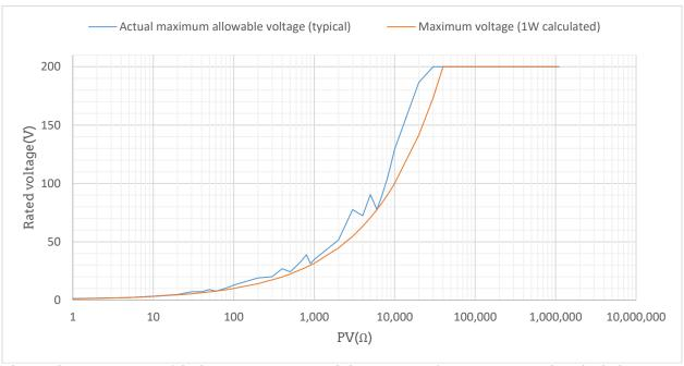
Above: The power rating of the base resistor is 1W, while in practice for most output values (PV), the power rating is usually between 1W and 2W. The user can use it according to the actual MaxU (rated voltage) returned from the serial port; for simplicity, it can also be always treated as 1W according to the rated voltage calculated by the formula  $MaxU = \sqrt{(PV^*1)}$ . It should be noted that the maximum applied voltage across the output resistor should not exceed 200V.
