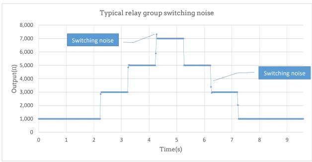
Above: The "output resistance noise" generated by relay switching occurs on the rising or falling edge, and is more obvious during some resistance switching. It should be noted that the relay switching algorithm of the QR10 is not specifically optimized, so in some cases, the output may be open or shorted for a short period (ms level).
